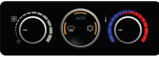
Blower Control Left: Climate Control Switch/ Right: De-Fog Switch Temperature Control
