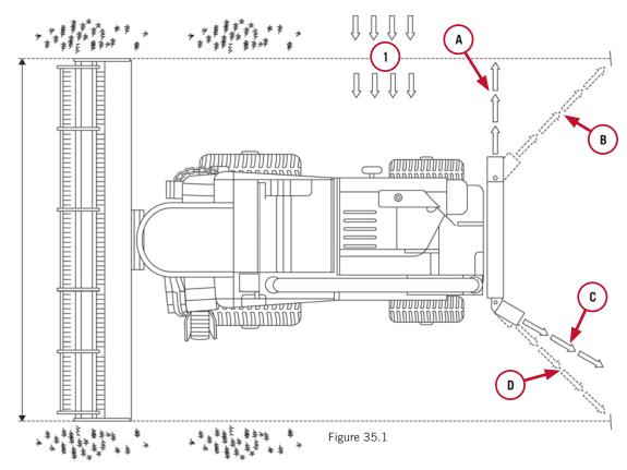
**NOTE:** Starting with model year 2016 and forward, the Axial-Flow combines will utilize adjustable distribution panels for spread control. The 3-sided chutes will serve as wind protection. For more information consult the proper operators manual.
