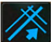
The next swath function (1) is only available in square headland mode in field swaths and in Multi-Swaths. The icon for the next swath function is visible underneath the custom map icon in the left-hand menu of a map.
