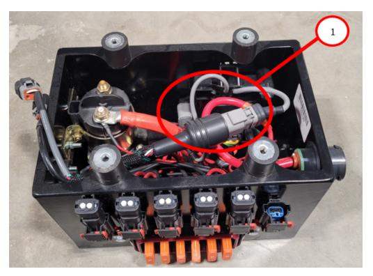
**Step 5:**Plug the 729818 harness into the SRM and PDM harness connection as shown.
