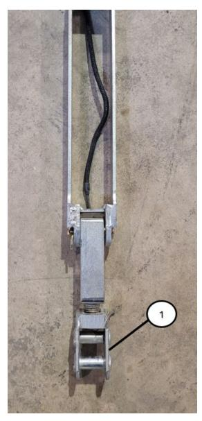
**Step 9:**Remove the cotter pin and clevis pin (1), then remove the down force sensor (2).
