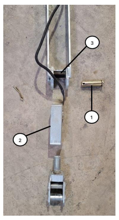
Note: Ensure the rubber depth spacer (3) remains in place between the down force sensor and depth control linkage when installing the new sensor.
