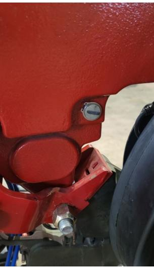
Step 13: Re-install the depth handle and set the depth appropriately.
